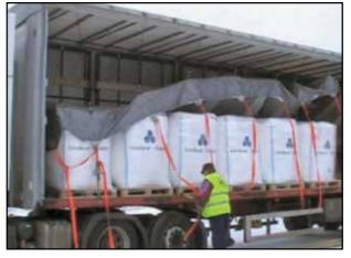
A suitable alternative system for load-securing.
