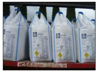
Not secured in a curtainsider – unacceptable.
