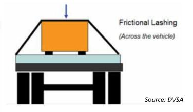
Relies on the lashings being as vertical as possible increasing the down force on the load and the friction between the load and bed of the vehicle.
