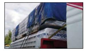
This load is shown with additional securing. An additional hammock strap and cross-strap was fitted after the vehicle had been stopped at roadside. This arrangement was adequate to restrain a load of this weight and to allow the truck to carry on.
