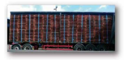
A light load with a difference. None of the pallet stacks exceed c.400kg, so internal straps are appropriate.
