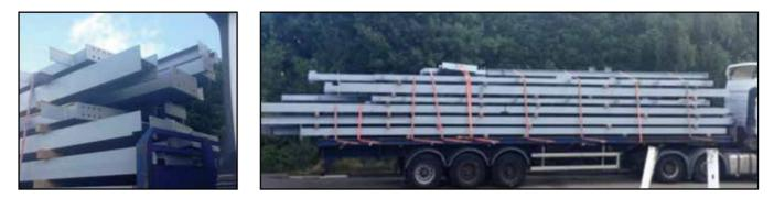
Examples of loads above the headboard which require additional securing, more than is shown in the pictures. Additional lashing is-required – both top-over lashing to increase downward loading plus additional lashing/support across the front of the load to prevent forward movement, possibly a temporary headboard or heavy-duty hammock/sail sheet.
